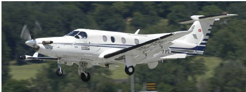
Pilatus PC-12 taking off with relay antennas and equipment installed
